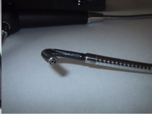
Close up of articulated objective tip
